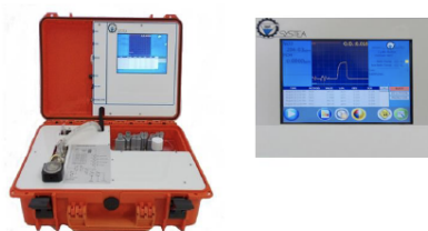
Fig. 2 - SMS modular automated measurement prototype with portable analyzer touch screen.
