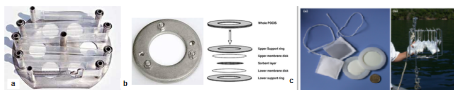
Fig. a. SPMD sampler; b. POCIS sampler; c.SPATT samplers
